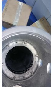
OTE sampling bottle with ball assembly removed to show the stainless steel springs that push up on the floating seal ring (not shown) to seal it against the rotating ball (i.e., the ball in a ball valve).
