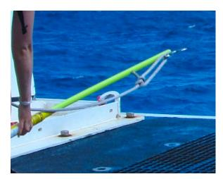
Telescoping fiberglass pole with Wichard mooring hook and line for attaching tag lines to the carousel during recovery.
