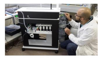
A pico-Fast<sup>®</sup> system has been acquired for pre-concentration of sea-water samples for trace elemental analysis using ICP-MS. The system is currently undergoing installation and validation for measurement of bioactive trace elements.
