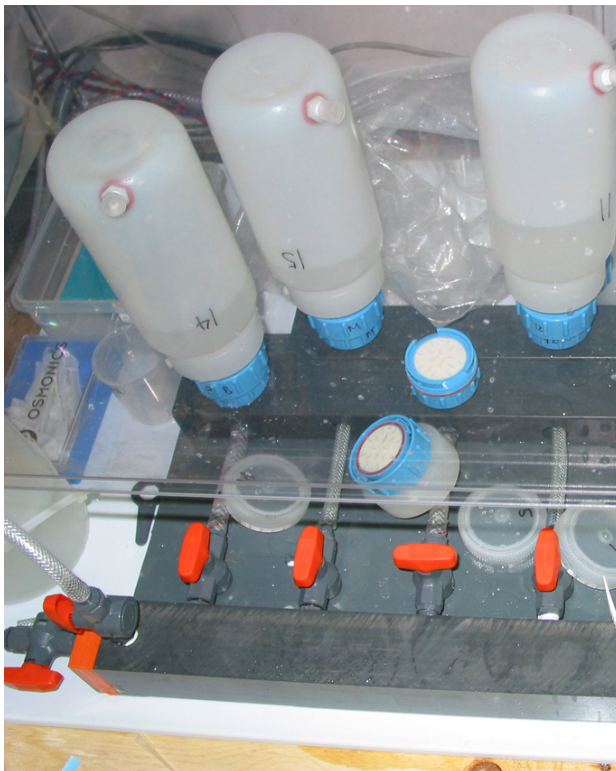
Figure 3. An example of a 1 L offline filtration method as used routinely on CLIVAR A16N, A16S, VERTIGO, and GEOTRACES IC expeditions. Pre-cleaned 1L LDPE bottles are modified with closing air vents at bottom. Sample is quickly transferred from the GO-FLO into the 1 L LDPE bottle which is then capped conventionally. Once returned to a Laminar Flow bench environment, the top is substituted for a tapered adaptor which has a mated 47 mm MFS filter holder with preloaded 0.45 \mu m Supor filter. The upstream orifice of the filter holder has been drilled out to twice standard diameter to minimize air-lock effects. Once samples are filtered under 25 to 40 mm Hg vacuum, they are transferred directly to sample bottles for further processing. Primary sample bottles and filter holders are reused after TM-clean DI water rinsing. More information available from J. Bishop ( jkbishop@berkeley.edu ) or Todd Wood ( tjwood@lbl.gov ).
