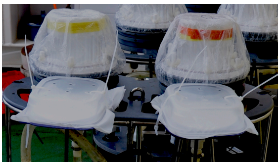
Figure 6: Dipped blank filter sets sandwiched between 1 \mu m polyester mesh, and deployed in perforated plastic containers that are attached to the pump with cable ties.
