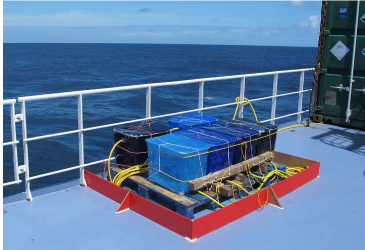
Figure 1. Incubators for the 6 different depths with adjusted light lifters (54%, 25%, 13%, 3%, 1%, 0.2%) as setup during the Geovide cruise
