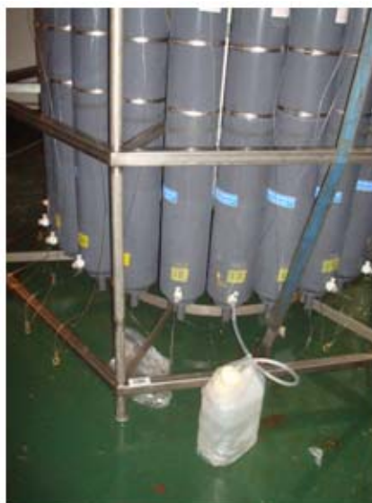
Figure 26: Sampling and filtration of seawater on board. The acid cleaned sample bottle was kept in two zip-lock bags and the sample was filtered directly from the Niskin bottle, which minimized the contamination from the ship.
