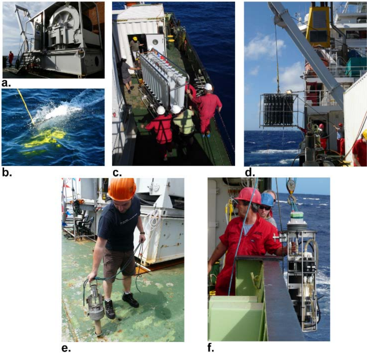
Figure 10. Equipment used during JC057: a) Kley France winch with mounted A frame, b) the towed fish used for underway surface sampling of seawater, c) the ultraclean all titanium CTD transported to its custom made cleanroom container for sampling, d) the high volume CTD25L during recovery, e) Leo Pena holding the mono corer used underneath the CTD25L to sample bottom sediments for Nd isotopes, f) the Chief Petty Officer Scientific Mick Minnock and Stephanie Owens deploying an in situ pump. Pictures a, b, d, e and f by Michä Rijkenberg, Picture c by Elizabeth Jones.
