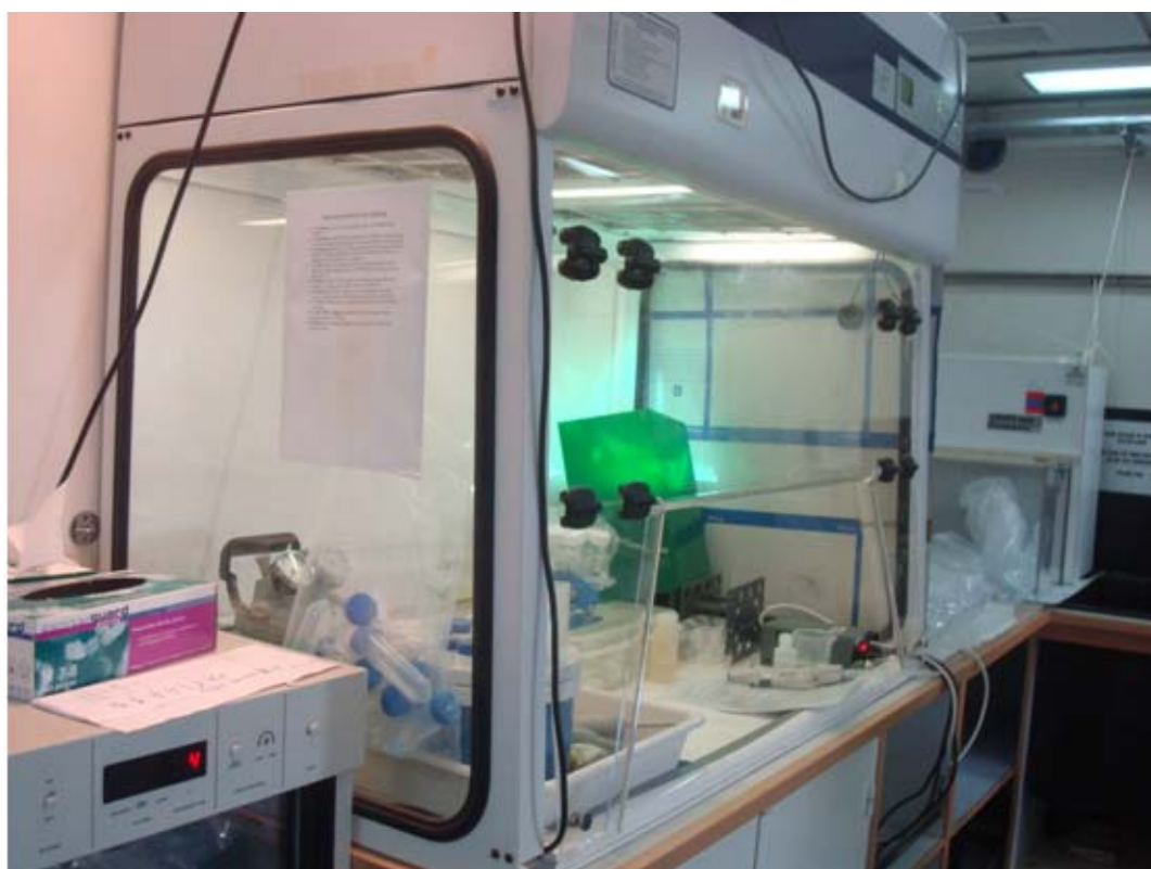
Figure 27: Fume hood in the chemistry lab aboard, where acidification of samples was conducted.
