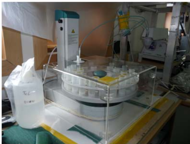
Figure 19. The voltammetric equipment with in front the sample changer. The electrode stand is mounted in a NIOZ home-made aluminium frame on a wooden board that is hanging in elastic bands, preventing scans to be disturbed by motions of the ship. At the left is a sample that was taken to test the influence of bacterial activity on the characteristics of the ligands. The sample is kept in the laboratory at room temperature to stimulate bacterial activity.
