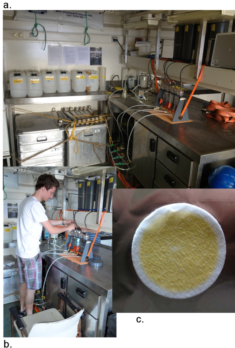
Figure 30) (a) Overview of the filtration system set-up. (b) Pim filtering the sea water in order to capture the phytoplankton. (c) A 47 mm GF/F filter after filtration of 10 L of sea water from the 25L CTD. The colour change from white to green/yellow/ brownish caused by the phytoplankton is clearly visible. White spots can be caused by grazers on the filter, such as salps. The filter can either be used for HPLC analysis or Chl-a absorption measurements.
