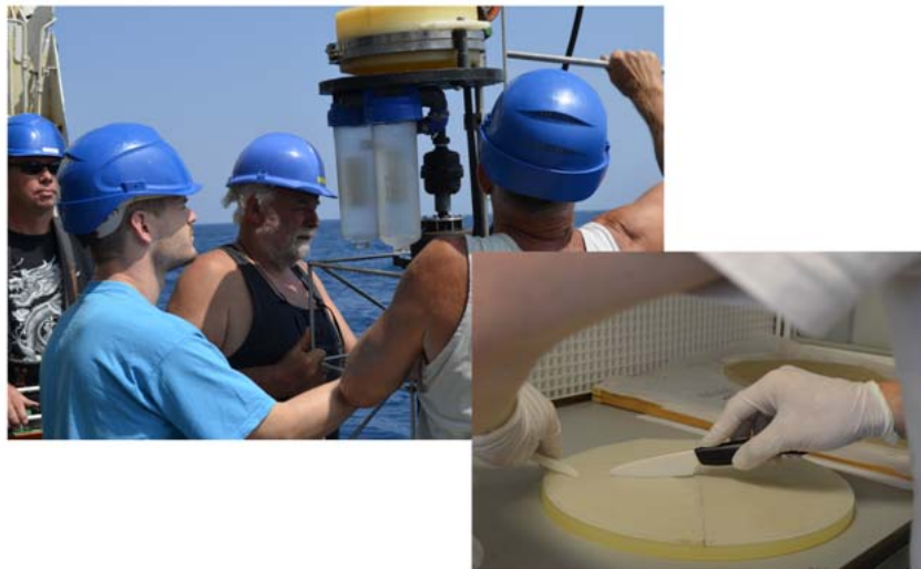
Figure 27. Cor, Matt, Jack and Sjaak handling the SAPS and on the right Matt sub-sampling a 293 mm polycarbonate 1 µm pore size filter.
