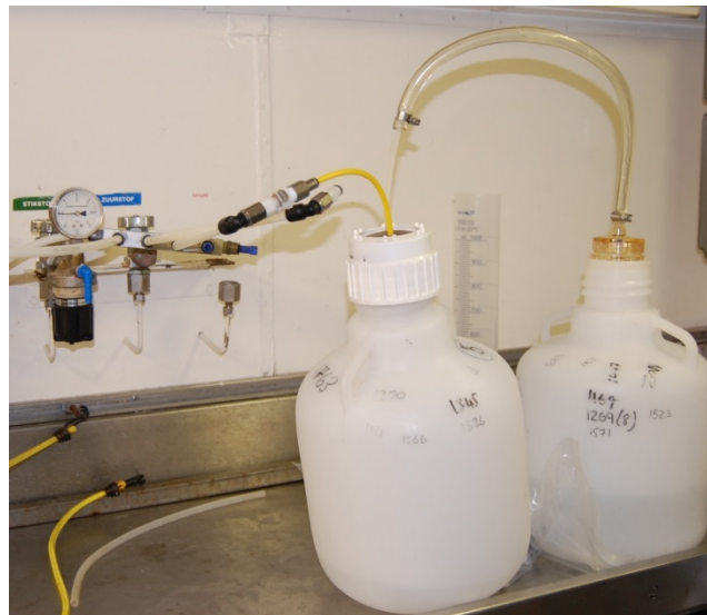
Figure 31. Filtration system used for the collection of particles at surface and deep chl-a maximum to measure Si isotopic signatures of biogenic silica during Leg 3 of MedBlack GEOTRACES cruise.
