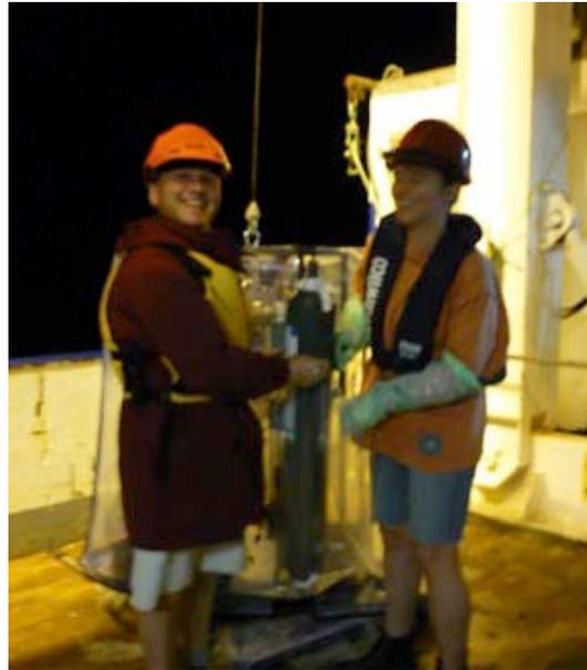
**Figure 1: Trace metal Rosette and Niskin Bottle. It is important to note that trace metal clean procedures were followed during all stages of the sampling process.**
