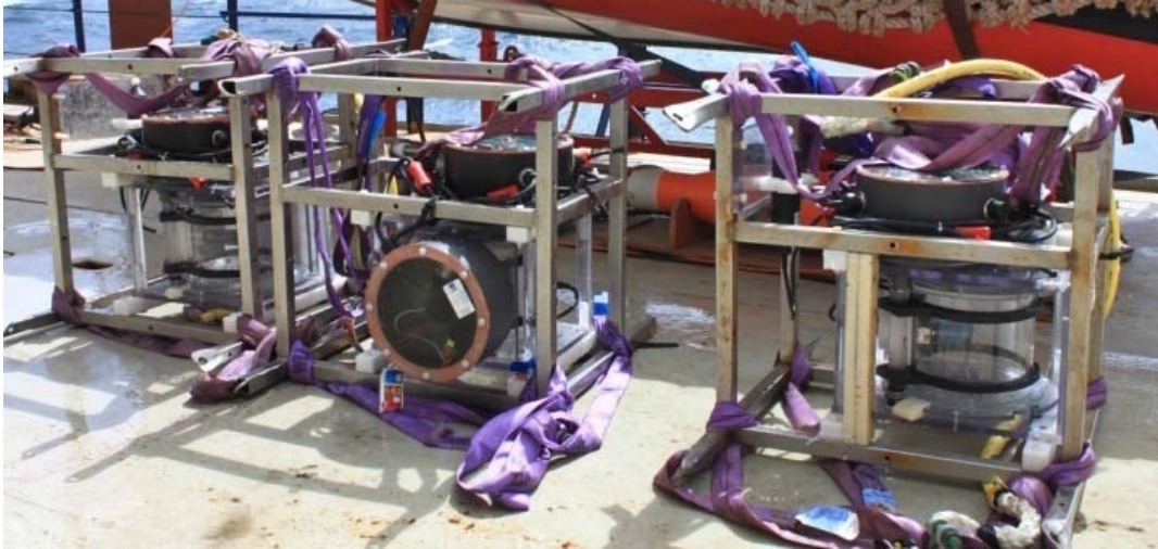
Figure 24 : IODA #1 / @DeepIodaV4 MSP version PP_2010_3_16 corr for 4330/ Optode Int 4330 373 / Optode ext 4330 120 / PAR # QSP 2200 – 50113 / QSL, SN:10434, microEins- teins/m2/s, dry calibration.
