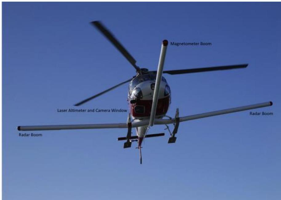
Figure 1.16. Configured survey helicopter with booms.
