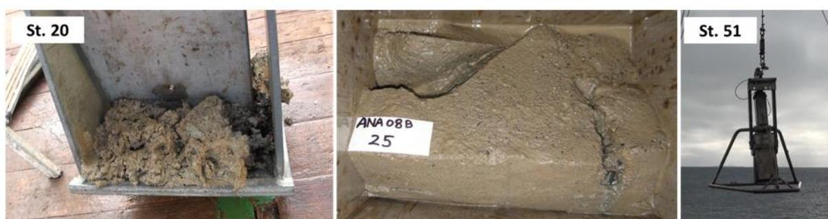
Figure 4.3. Box coring at St. 20, 25 and 51 was performed unsuccessfully due to high gravel contents.
