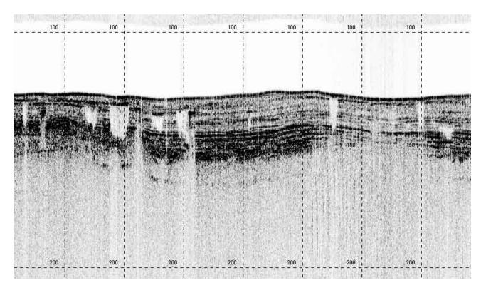
Figure 7. Acoustic blank zones underlying relatively flat seafloor northeast of Heard Island (see Figure 4; stations 26, 32, and 48-51 were undertaken in this area, which is an acoustic plume field), as imaged on raw SBP120 data. Water depth averages ~85 m.
