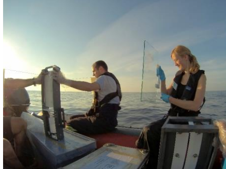
Figure 3. Two 'clean' sampling devices were used when sampling from the rubber boat, to characterize the chemical (trace metals, organic matter) and biological (pico and nano-plankton)
