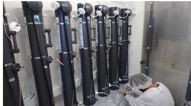
Clean rosette used in PEACETIME (left) Deployment preparation (right) Subsampling from clean rosette bottles respecting trace metal clean techniques (bottle were removed from the rosette and subsampling in clean container).
