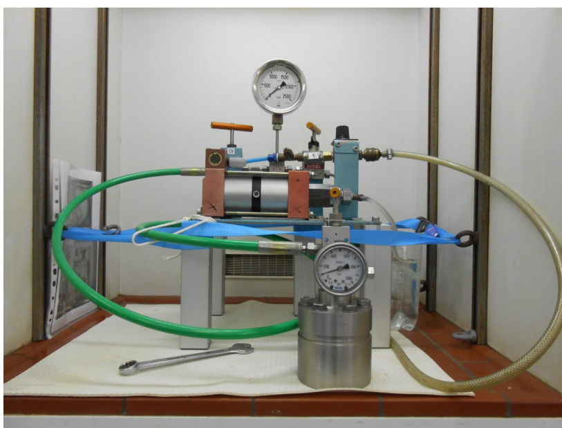
Fig. 9.1 Pressure generating system to expose deep-sea nanofauna at different hydrostatic pressure.
