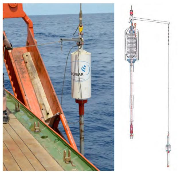
**Fig. 6.14:** Operation of the GEOMAR piston corer during SO-225 (right) and schematic diagram of the split-piston corer from Fa. Marinetechnik Kawohl.
