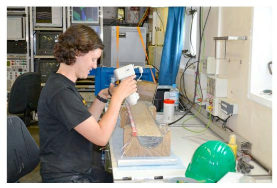
Fig. 6.19: Color scanning the SO-225 sediment cores.
