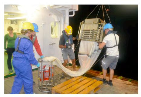
Fig. 6.6: The AWI multinet deployed during SO-225.
