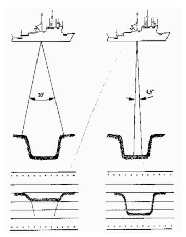
**Fig. 6.7:** The extremely narrowed beam of the ATLAS PARASOUND of 4.5° compared to a conventional echosounder system and a beam angle of 30°. The ATLAS PARASOUND even resolves small-scale bottom structures and offers a deeper penetration of up to ~150 m into the seafloor (ATLAS Hydrographic).
