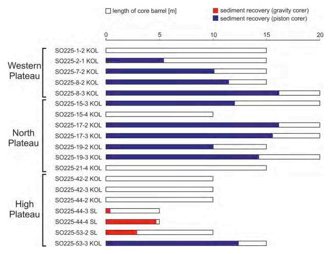
Fig. 6.15: Length of core barrel and core recovery of piston and gravity corers.
