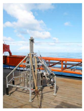
**Fig. 6.12:** GEOMAR multicorer with Kawohl-Marinetechnik Deep Sea TV-Camera system. Technical specifications: Height: c. 2,250 mm, diameter: c. 1,900 mm, weight of head: c. 180 kg, weight of framework: c. 465 kg, number of tubes: 12, diameter of tubes: 100 mm.
