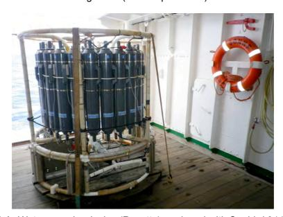
Fig. 6.1: Water sampler device (Rosette) equipped with Seabird 911 CTD.
