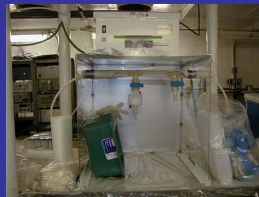
Clean bench with filtered and unfiltered clean water taps from fish/pump supply
