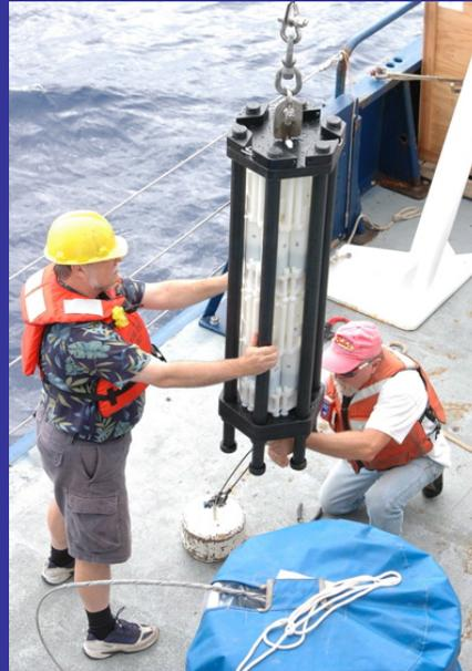
Ed Boyle's MITESS samplers. The vane sampler on the left is used to collect an individual smaller sample. The sampler on the right is used to collect multiple samples to either provide a larger volume or used with a timer to collect at multiple depths. Funding for participation is pending.
