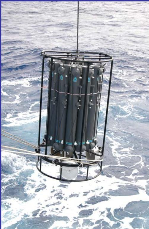
Bill Landing and Chris Measure's rosette system of 12 each 12 liter GO-Flo samplers with their clean conducting cable used in the CLIVAR program. This system is limited to the upper 1000 meters. It was shown in the SAFE program to be able to take clean samples for iron. There are still some problems for zinc.
