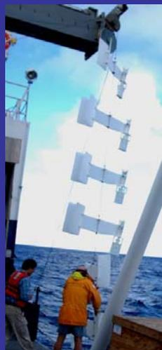
Jingfeng Wu's sampler based upon a modification of the original MITESS ATE/vane sampler that Ed Boyle developed. Funding for participation is pending.
